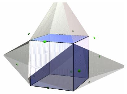
Figure 2 – VBAP 16-loudspeaker arrangement for a six-sided CAVE.
